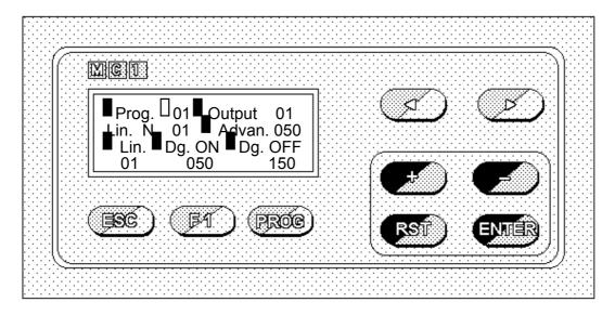
Send the blinking cursor to 'Prog.' field and press **F1** for over 3 seconds to enter in the **Parameters Edit** page.
