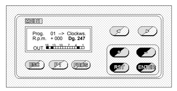
By pressing **F1** for over 3 seconds and by introducing the access code, the display shows:
