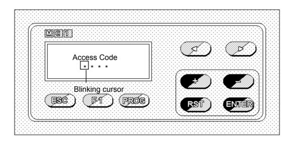
First of all, Access Code (Password composed of 4 key sequence) must be correctly introduced.
