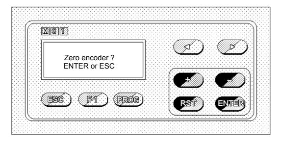
Press **ESC** to cancel the procedure or press **ENTER** to confirm the calibration: automatically the encoder position will be equal to 000.
