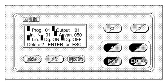
Press **ENTER** again to delete the sequence; otherwise press **ESC** to cancel the deleting procedure.
