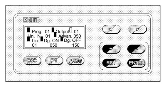
Send the cursor to the 'Output' field (blinking cursor will be near it). By pressing **RST** for over 3 seconds, the display shows:
